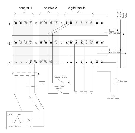
Wiring example for pulse encoder (5 V)
