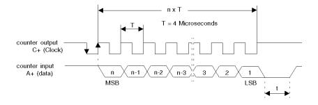
Each clock signal edge triggers the transmission of a data bit. The clock signal frequency is specified by the module and amounts to 250 kHz.
