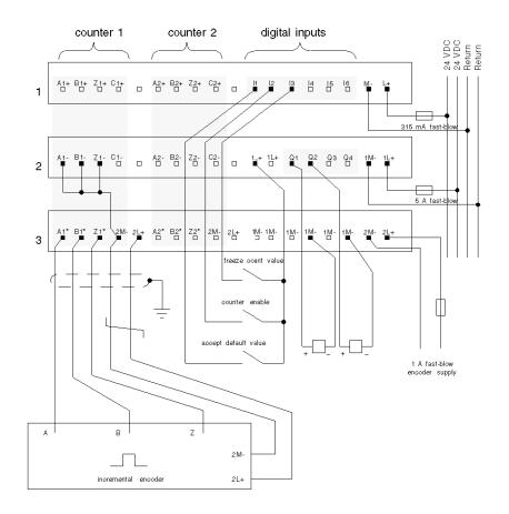
Installation for use as 24 V pulse encoder for A, B, and R line
