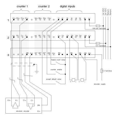
Installation example for absolute encoders with actuators
