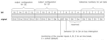
1 = inactive (to be used with encoders with 24 V single ended signals)
