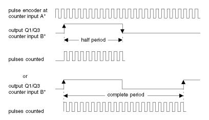
If no external clocking signal is available, digital outputs Q1/Q3 can be configured as frequency outputs. However, as the outputs are only available at 24 V level, the corresponding output Q1/Q3 must be connected with the 1M to counter input B<sup>\*</sup> and B-.
