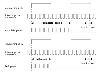
**NOTE:** Half period means the measurement of a series of pulses from positive to the next negative edge.
