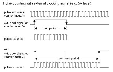
**NOTE:** When an external clocking signal of a 24V level is used, the external clocking signal must be connected to counter input B\*.
