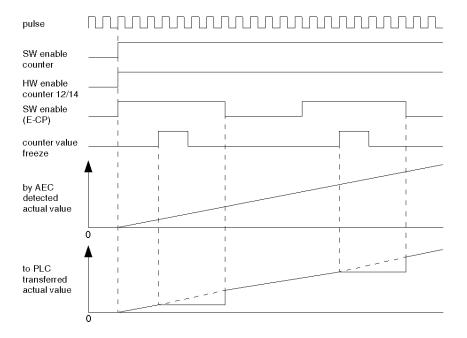
Pulse diagram of freezing counter value
