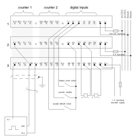
Installation example for pulse encoder (24 V)
