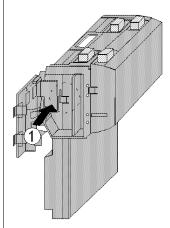
Result: The locking tabs on each side of the option adapter slide inside the I/O base and out through the locking slot. The 12-pin ATI connectors on the two units are mated to each other in the process.
