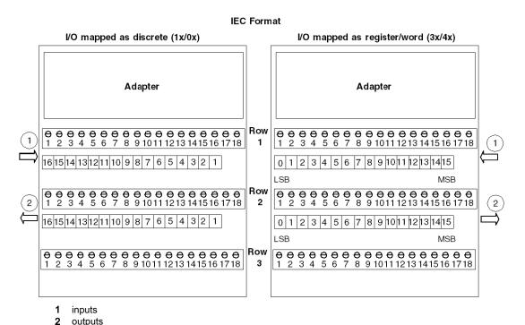
The figure below shows how data is mapped on the I/O base with a 984 Ladder Logic Compliant adapter. When the I/O is mapped as discrete points (1x/0x), the MSB is assigned to Pin 16 and the LSB is assigned to Pin 1. When the I/O is mapped as a word or register (3x/4x), the MSB (bit 15) is assigned to Pin 1 and the LSB (bit 0) is assigned to Pin 16
