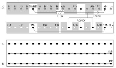
**NOTE:** AGND and DGND are connected at a single point inside the module. External digital inputs must be returned to the DGND terminal. External analog circuits must be returned to AGND terminals.
