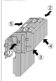
Once snaps 1 and 2 have been disengaged, use the screwdriver to release snaps 3 and 4 on the front of the assembly.
