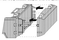
**Result:** The locking tabs on each side of the Processor Adapter slide inside the Option Adapter and out through the locking slot. The 12-pin ATI connectors on the two units are mated to each other in the process.
