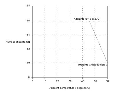
At 60 degrees C and maximum input voltage, the number of points allowed ON is 10.  $\,$
